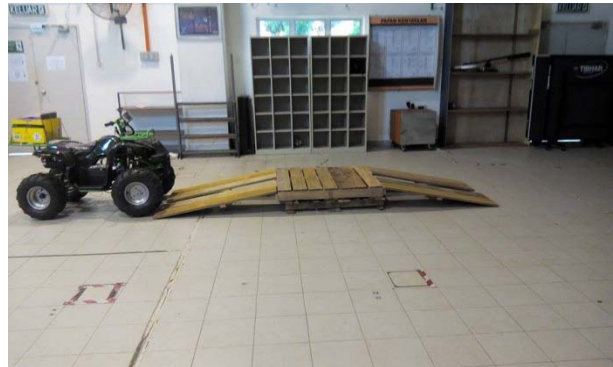
Fig. 11. ATV testing for climb the obstacle
